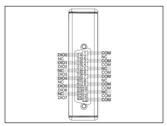
Figure 1. NI 9401 Pin Assignments
